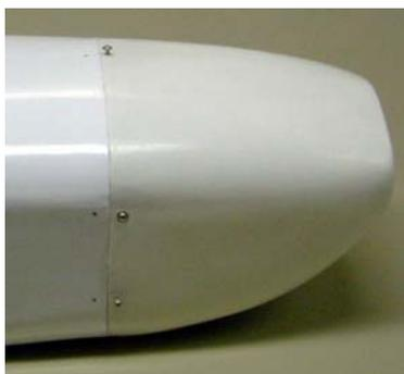
2. Retrieve the cowl and slip it over the 5 cowl mounting blocks. Position the top center of the cowl along the edge of the foredeck, and with the edge fitting over the recess and flush with the foredeck, apply a piece of tape to hold in place. (Don't cover the dot!)
