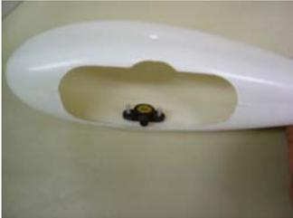
6. Secure the wheel pant, and retaining collar so that the wheel spins freely, and the wheel pant is snug to the axle shaft.
