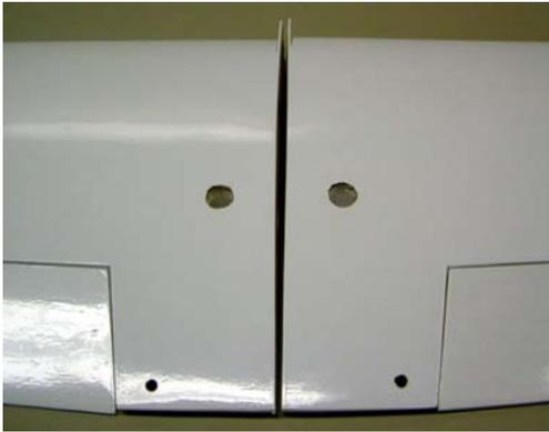
iron and open the two  $\frac{1}{4}$ " (6mm) wing mounting bolt holes (top and bottom) and the two  $\frac{1}{2}$ " wire exit hole located on the top of the wing. (The servo wires enter into the cabin space from the top side of the wing.) If using the razor knife, you'll get better results if you cut on the downward stroke – pushing the covering against the underlying wood for support as you cut.
