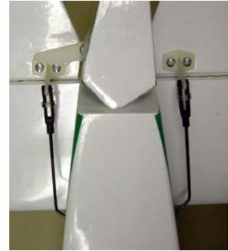
10) To mount the elevator servo, center the pushrod in the cockpit so that it is near the center of the fuselage. (You can see that if you move it side to side you will affect the
