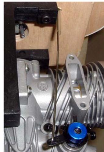
24) Slide the connector/servo arm over the throttle wire and position the servo arm on the servo output shaft/splines so that full travel will close the throttle.
