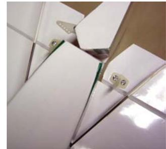
9) We are going to make a shallow 'Z' bend in the rod. The purpose is to convert the 'Y' so that it pushes parallel to the aircraft centerline, and have the clevis connect with the control horn squarely. (see pictures and read below)
