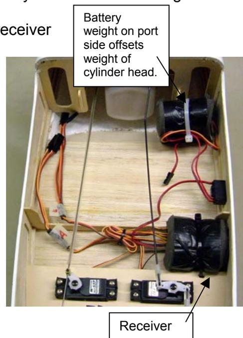
Battery weight on port side offsets weight of cylinder head.
