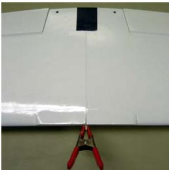
approximately 4 3/4" (120mm) at the wing tip corner, where the aileron meets the tip.
