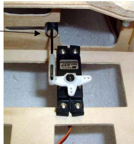
11) Turn your transmitter on and plug the servo into the receiver. Position the servo arm so that at idle position the servo arm is at right angles to the elevator pushrod. Cut off the other servo arms as necessary to prevent interference with the pushrod action at extreme travel. Turn the radio off, transmitter last.
