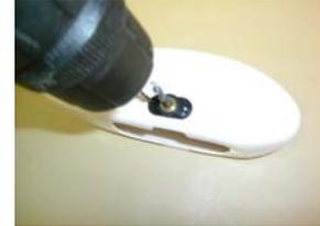
4. Assemble the bracket bolt and nut as shown in the picture in step 1 above. Position the bracket flat side against the inside of the wheel pant, and secure using two sheet metal screws (#20) from the outside. (Using the drill shank again helps with alignment.)
