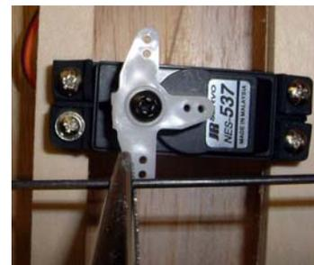
13) Double-check the position of the elevators. Adjust the clevises as necessary to align them with the stabilizer and each other.
