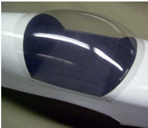
Trim the canopy to fit the fuselage using the molded in lines as a guide. Cut outside the lines on your first pass and test fit. We like using a pair of aviation or metal tin snips to do this job. Aviation tin snips are offset to one side, allowing the material to pass alongside the tool while cutting, and they have the power to make the job easy. (They come in left and right hand versions.) Good stout scissors are your next best tool.
