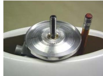
5) Using a pencil through the cowl air inlet, while pressing down on the shaft to prevent the engine from moving, mark the accessible corners of both the upper and lower engine mounts against the plywood.
