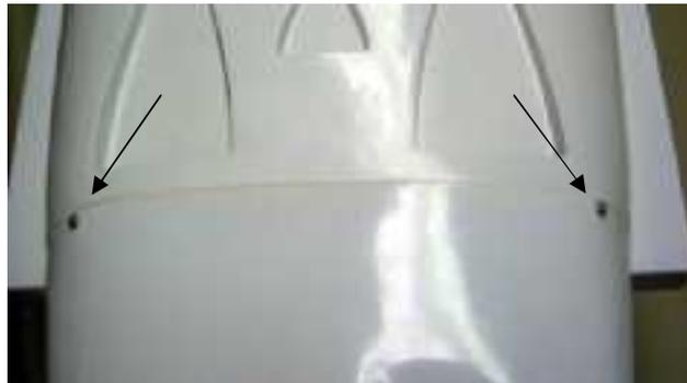
3. When comfortable with the fit, drill a  $5/64"$  (2 mm) hole at each dot,
