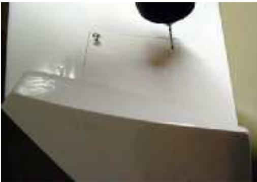
13) Position the winglet into place on the wing and drill four 1/16" holes at the pin punches, through the winglet plate into the plywood in the wing. Watch to be sure you do not pinch wires as you assemble the winglet to the wing.
