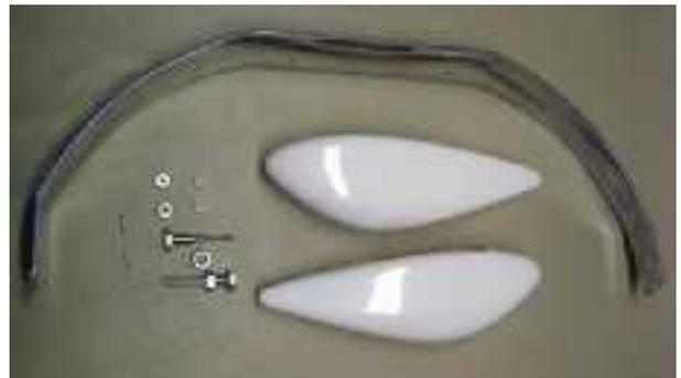
2. When installed, the landing gear sweeps forward, Fit the recess molded into each wheel pant to the correct end of the landing gear and mark the location of the main axle hole and smaller retaining hole. Our 'manual' model needed the ends of the gear trimmed to the correct
