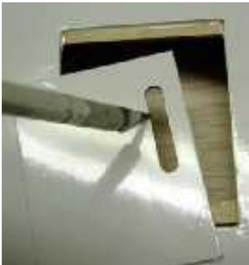
(Don't use the soldering iron trick, as it will show the melted edge where it would be visible from the bottom side of the plane. When cutting with the razor knife cut on the 'push' stroke – this will give a cleaner edge.)
