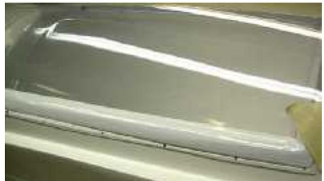
with the aft end of the cockpit cover. Mark the canopy along the top edge of the fuselage at the sides, and cut the bottom edge of the canopy so it will just touch the fuselage when it is attached to the cockpit cover.
