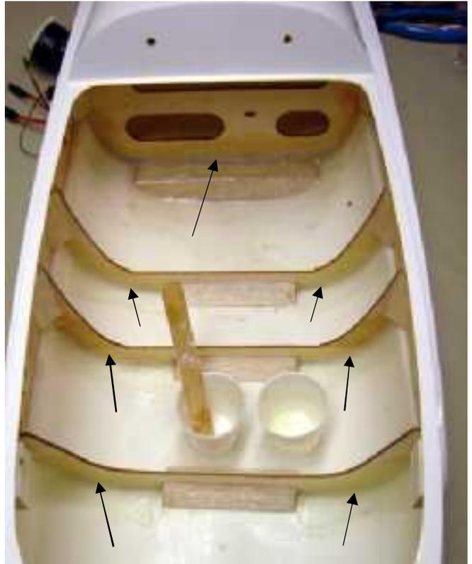
Congratulations! You've just done a technique of reinforcing corner joints (with flox and glass tape) that is identical to the way it's done on the full scale Velocity.
