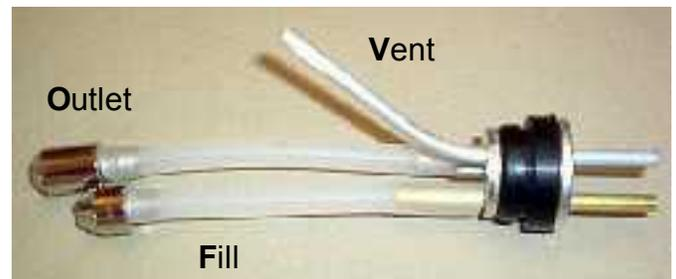
fuel pickup piece enters straight in. Mark the large outside metal disk with (O)utlet and (V)ent and (F)ill so you know which tube is which. Do not tighten the plug screw yet.
