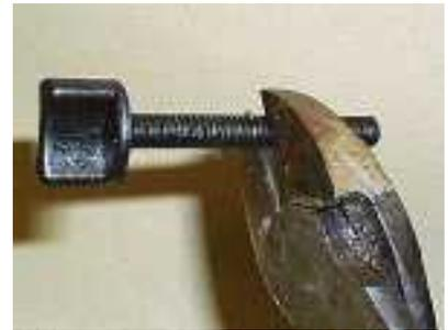
5. Test fit the bolts into the wings through the sides of the fuselage into the holes provided. They will line up with blind nuts already installed in the wings.
