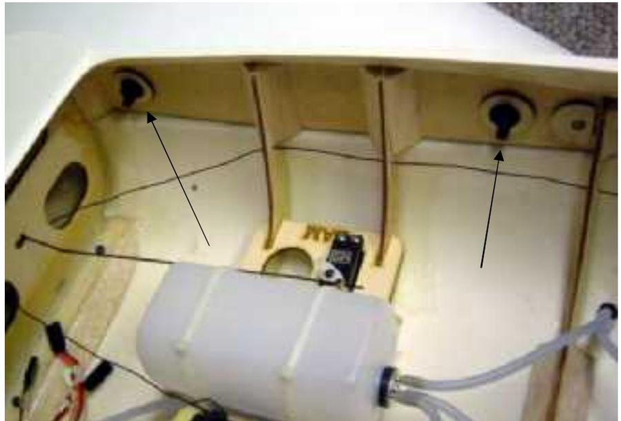
carry-through may be just a little too long. The cutting tolerance on this tube was designed to be on the 'plus' side to ensure proper seating of the tube at the ends inside the wing – where there is a plywood doubler surrounding the tube. Trim the length of the tube if necessary by an amount equal to the width of the gap.
