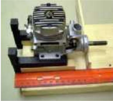
3) Place the motor mounts on a work bench or piece of wood so that the short legs overhang, and raise the mounts enough so that when the motor sits on the rails, it will not bottom out on the bench.
