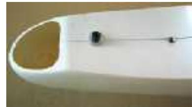
4. Install the stabilizer using the M4 bolts and washers. (See picture above)
