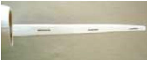
9. Remove the rudder and the CA hinges from the rudder and trim away the covering and drill the slots for hinge bonding into the rudder.
