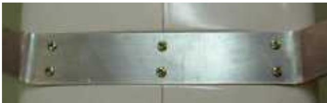
Use (a # 11) M3.5 x 20mm bolt as you drill each hole to help hold position. Remove the landing gear and drill out the holes to 7/32" (5.5 mm)
