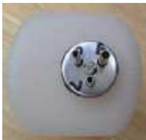
2) You will need to gently bend one long piece of tubing to reach up to the inside top of the tank to create the vent line. The short fuel pickup piece enters straight in. Mark the large outside metal disk with (O)utlet and (V)ent and
