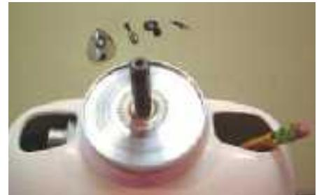
5) Press down on the engine shaft to prevent the engine from moving and mark the corners of both the upper and lower engine mounts against the plywood.
