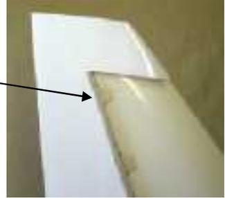
8. Using the hot soldering and/or razor knife, prepare the slot areas in the center line of the fin to accept the hinges. Finish hinge preparation by drilling a 1/16" hole in the center of each slot.
