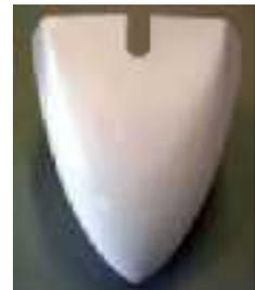
b. Mark the bottom of the nose cone where you will cut away clearance for the nose gear.
