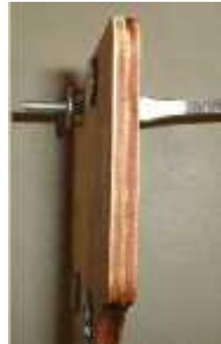
6) Retrieve the six (6) 3/16" washers from the U.S. Pack. Secure the engine mounts, short legs up, by using the (4) M4 x 25 mm (#12) bolts into the firewall blind nuts.
