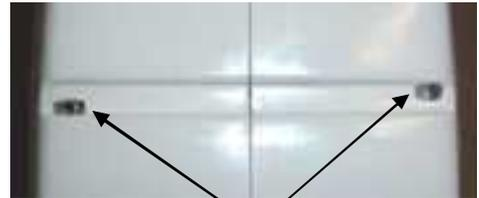
7) Trial fit the main gear legs into the holes with the short legs entering the holes. You will need to radius the inside edge of the hole towards the center line of the model so that the leg will sit flush on the bottom of the fuselage. (A Dremel<sup>tm</sup> tool or small round works well here.)
