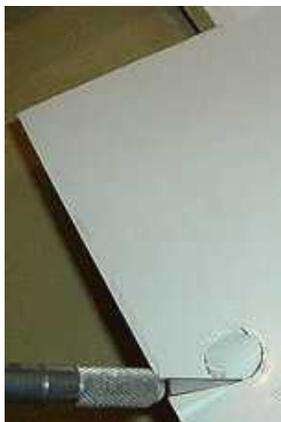
mounting bolt holes on the trailing edge of the wing to expose the blind nuts. Also open the two 1/2" wire exit holes located on the bottom of the wing.
