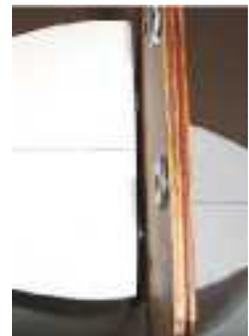
8) Trial fit the firewall with the 6-32 socket head cap screws (#2) and No.6 washers. Note that the lower M4 blind nuts will contact the fuselage. This is normal and allows enough space to slip the wing in place if you don't have an engine with a muffler that overhangs the trailing edge.
