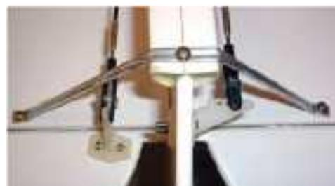
rudder and elevator horns. They should be in line with the clevis on the pushrods. The row of holes should line up with the hinge line of the surfaces. Use the nylon backing plates and 2mm machine screws (#20)
